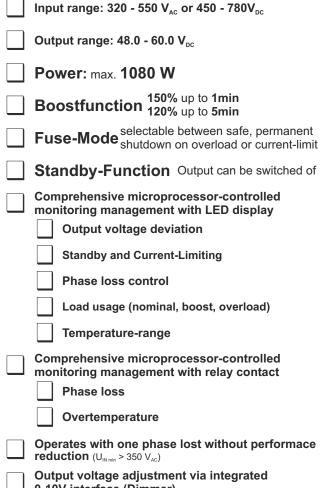
0-10V interface (Dimmer) Parallel operation possible, short circuit proof, overload
