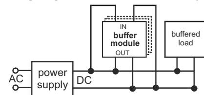
wiring diagram with buffered and un-buffered-load
