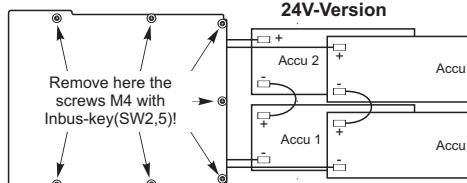
Reverse polarity of battery causes the damage of the device and is not repairable. This leads to termination of warranty.
